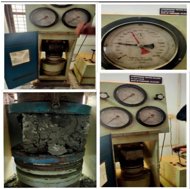
FIG 14. CTM-Compressive test done on the RAC
