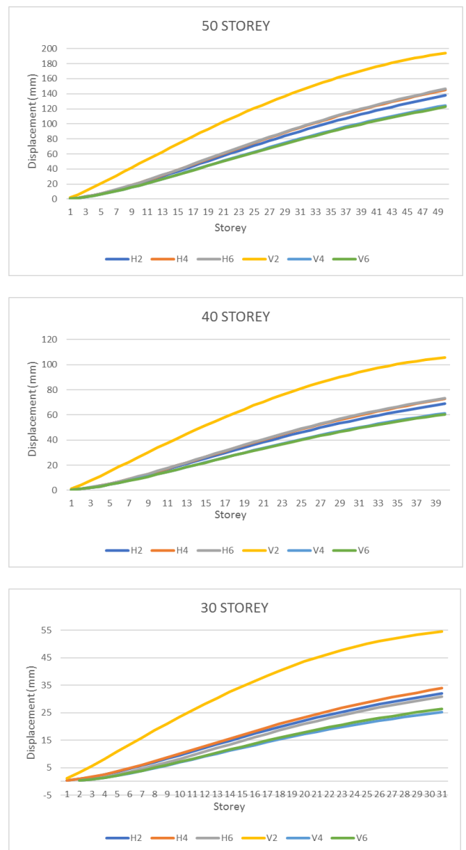
Fig-5: Displacement of various hexagrid module
