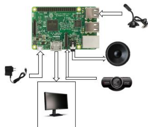
Figure 1.2: Connection between Raspberry Pi and I/O Devices.
