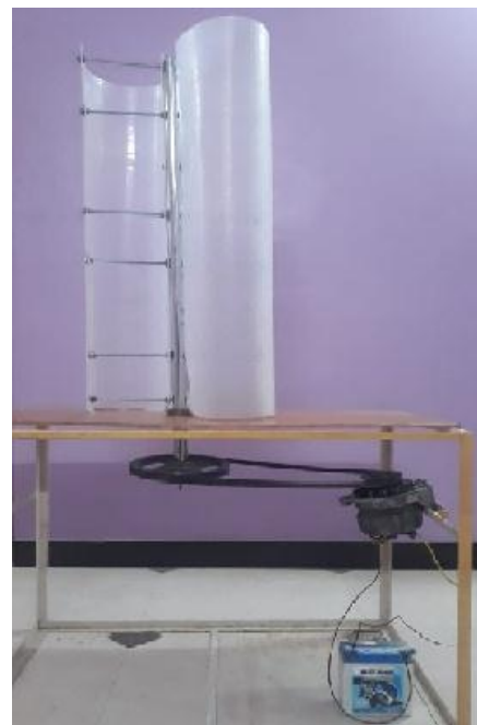
Fig -6: Experimental Setup for Vertical Axis Wind Turbine Prototype
