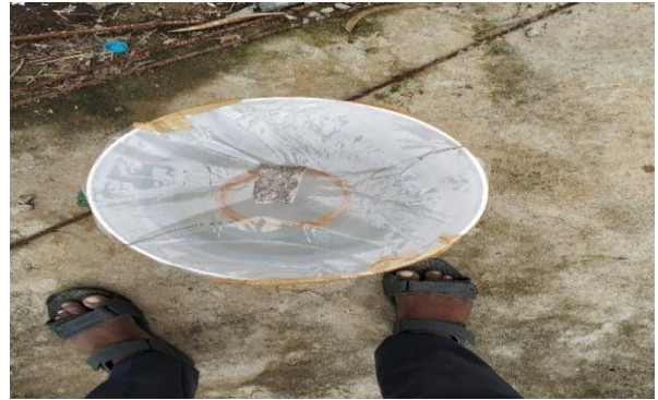
Fig: 6: Covering Bucket and placing a stone
