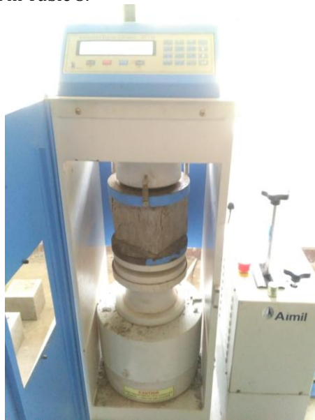
Figure -3: Cubes kept under Compression using Digital compression testing machine
