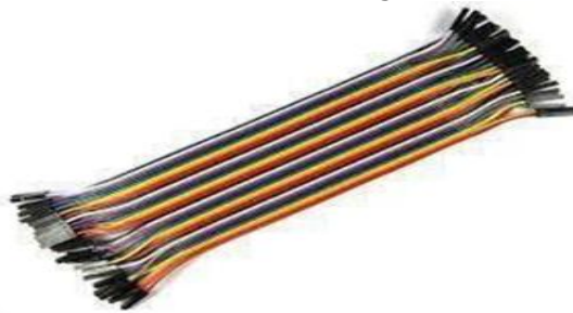
Fig -2: Jumper Wires
