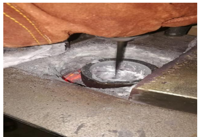
Figure (9) stir casting inside a furnace
