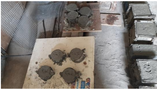
Fig 4- Casting of specimen
