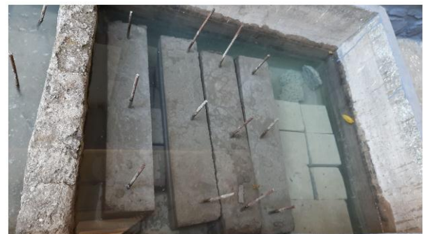
Fig 3- Curing of Beam
