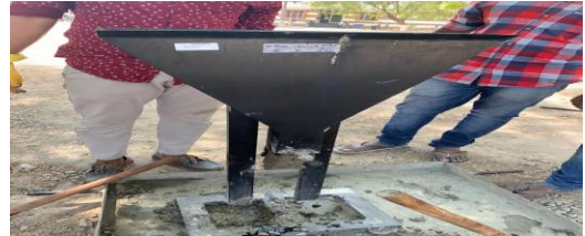
Fig 3.8.2 Concrete in V - funnel
