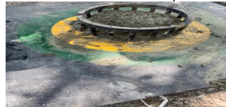
Fig 3.8.6 Concrete in J Ring
