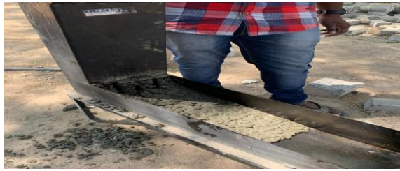
Fig 3.8.8 Concrete in L – box
