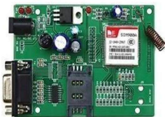
Figure 2.2 GSM Module Computer use AT Commands to Control Modem
