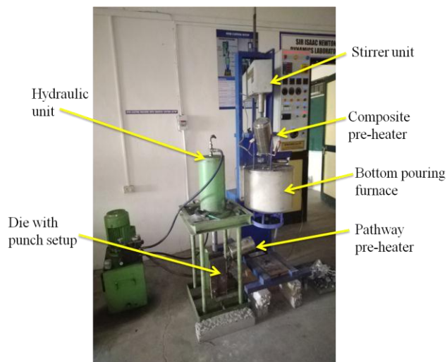
Fig -1: Squeeze casting machine set up
