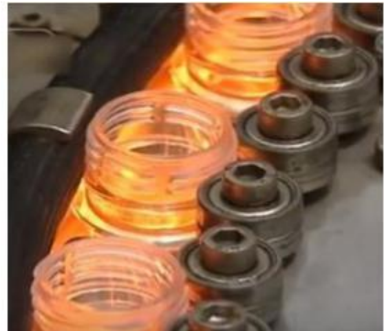
Figure 8: rotary pre-heater with bearing
