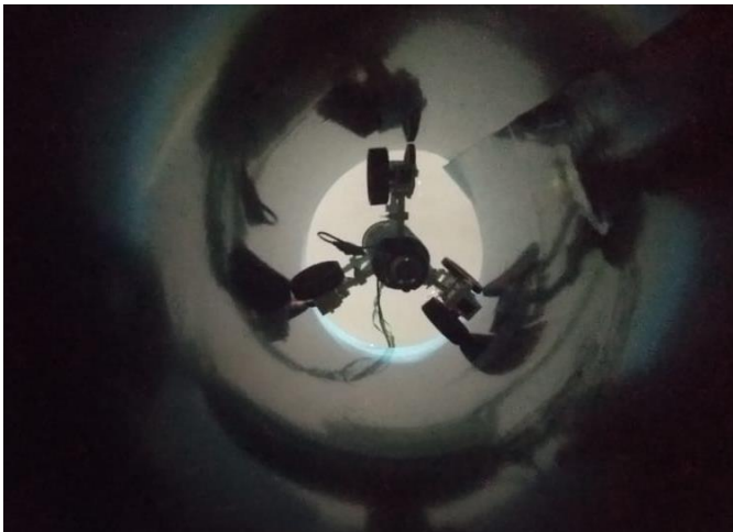
Fig -23: Robot moving inside the pipe
