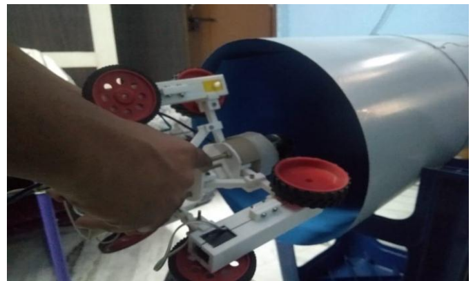
Fig -22: Inserting the robot inside the pipe
