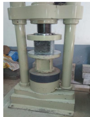
Fig -15: Compression testing on cube
