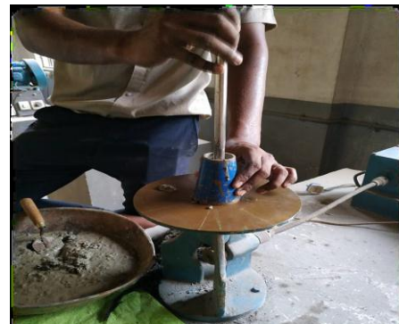
Fig-10: Compacting the mould
