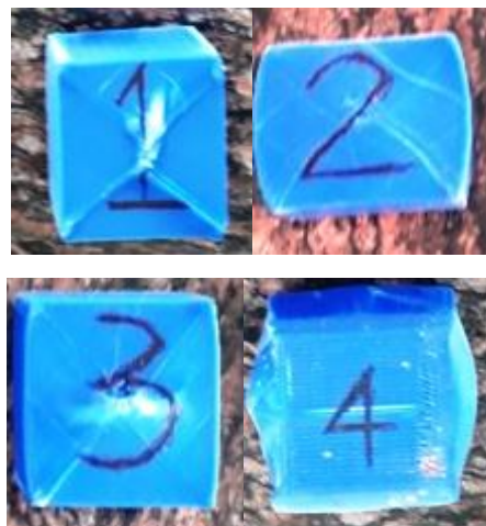
Figure Deformed Specimens after Compression Testing
