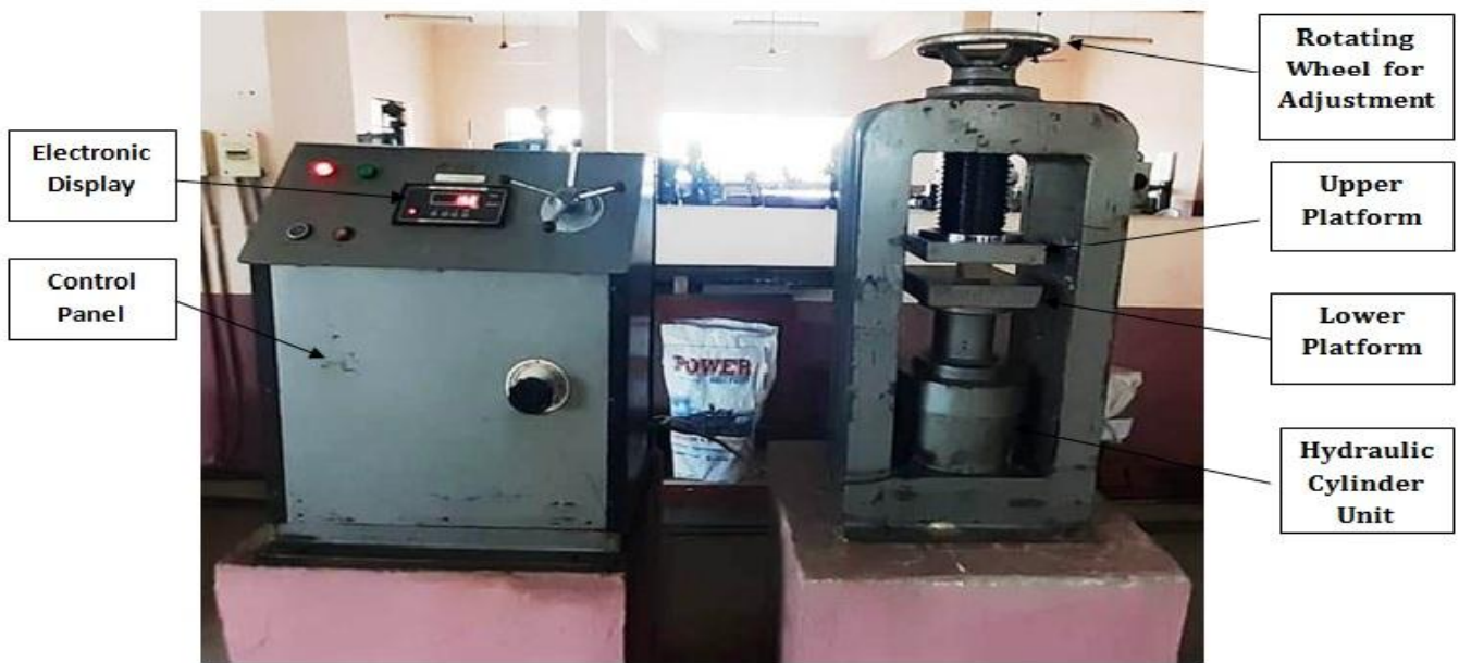
Figure Compression Testing Machine Experimental Setup
