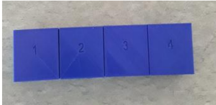
Figure - 4 FDM Printed ABS Specimens
