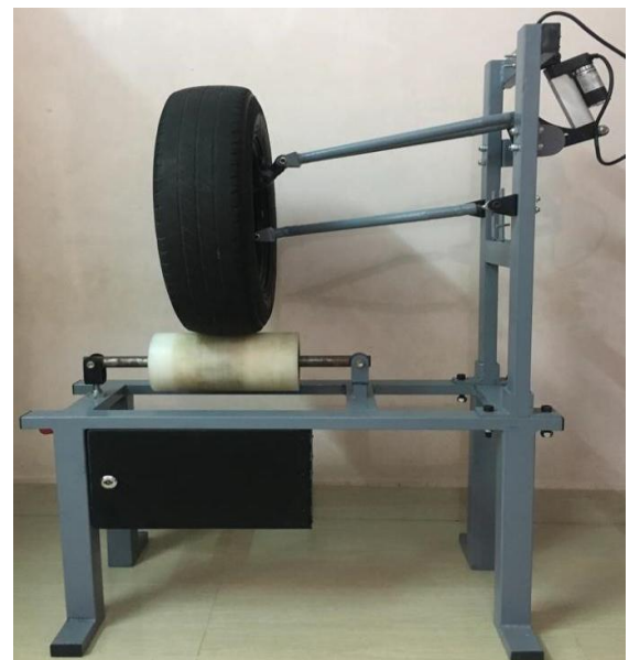
Fig -14: Fabricated Quarter model suspension test rig.
