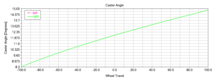
Fig -3: Plot of Caster Angle vs Wheel Travel in ADAMS
