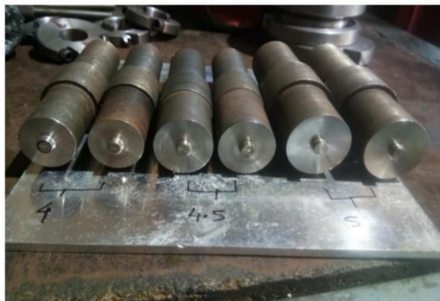
Fig. 5.2 FSW tools with different diameters
