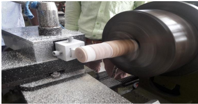
Fig-2: Cutting force analysis in lathe machine and lathe tool dynamometer.
