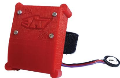
a) Exterior design: OperaBLE with pulse sensor
