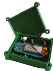
b) Interior design: OperaBLE with accelerometer
