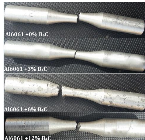
Fig.3. Fatigue Failure Specimens
