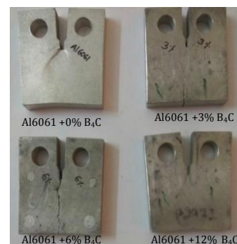
Fig.4. Fracture Failure Specimens
