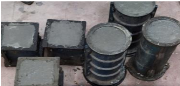
Fig-2: Casting of specimen
