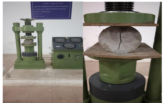
Fig-7: Splitting tensile strength test
