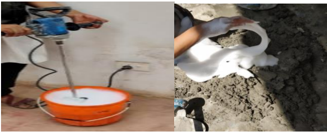
Fig -1: Foam preparation and mixing of it by pre-foaming method
