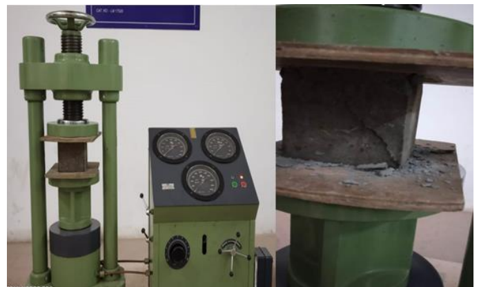
Fig -5: Compressive strength test
