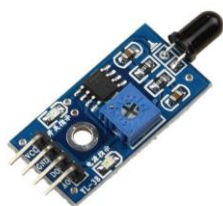
Fig 3.2 Infrared Flame Sensor
