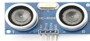
Fig 3.3 Ultrasonic Sensor Module HC-SR04
