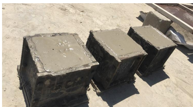
Fig -3: Casting of moulds
