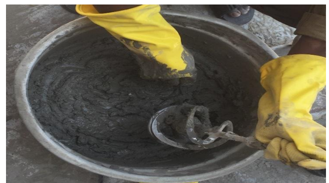
Fig -2: Preparing cement slurry
