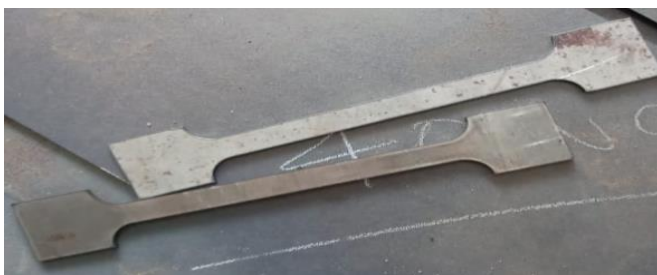
Fig.3 Cold form steel before coupon test
