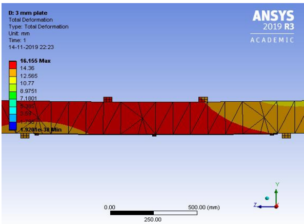
Figure.15 Total Deformation FOR ULTIMATE FAILURE LOADING:
