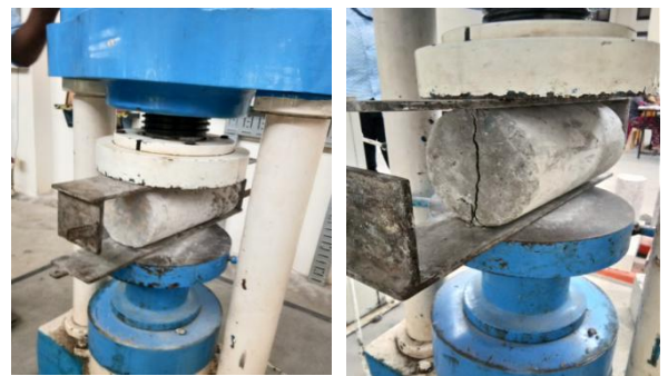
Fig.2 Split tensile test on Cylinder before and after loading
