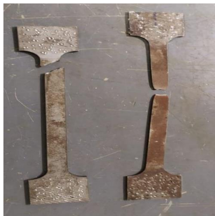
Fig.4 Cold formed steel after coupon test
