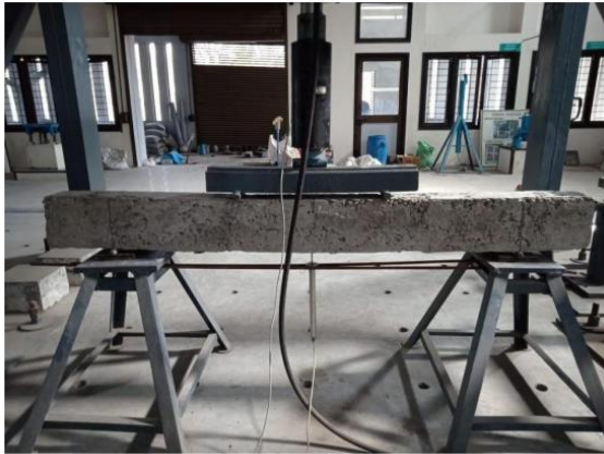
Fig.18 Testing of beam on Two-point loading frame
