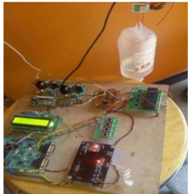
Fig 2: mode of intravenous flow monitoring system
