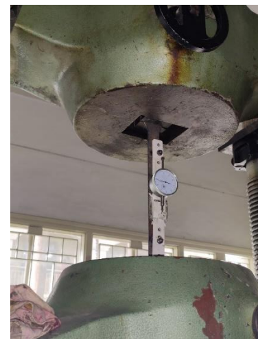
Fig 1. Tension Coupon Test Setup
