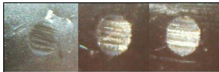
a) Ball One (b) Ball Two (c) Ball Three Fig-7- Scar images for sample W1 (SAE 5W30 base oil)
