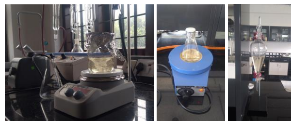
Fig. a Heating and stirring the coconut oil with catalyst
