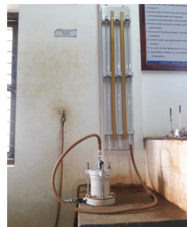
FIG-4: Falling head permeability test
