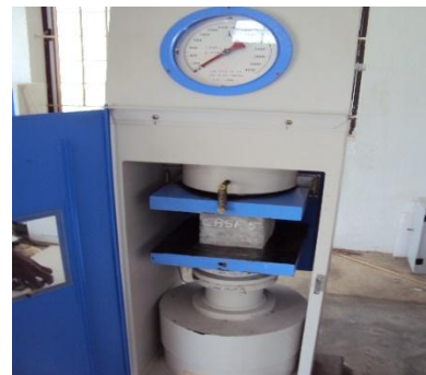
Fig :3 Experimental Setup for Testing of Cube Specimens
