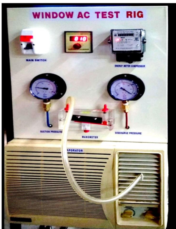
Fig 2.2 - Window AC Test Rig
