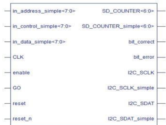
Fig -7: Pin Diagram of I2C [6]
