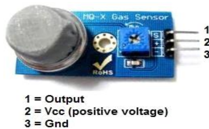
Fig -4.1:SMOKE SENSOR
