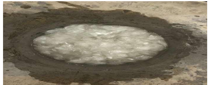
Fig -3: Placing 2% Polypropylene in Water Before Mixing
