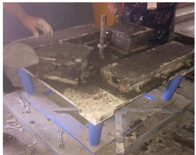
Fig -6: Placed Under Vibrating Machine to Settle
