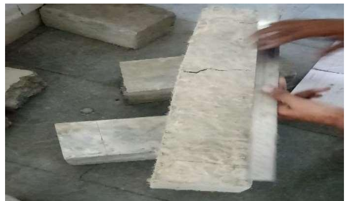
Fig -23: Failure of Specimen After Loading
