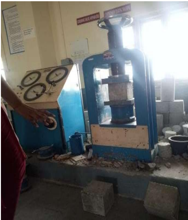
Fig -21: Testing of Cube Specimen After Curing
