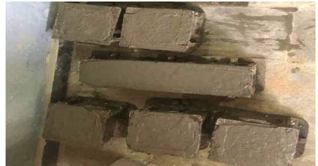
Fig -4: Casting Cubes
