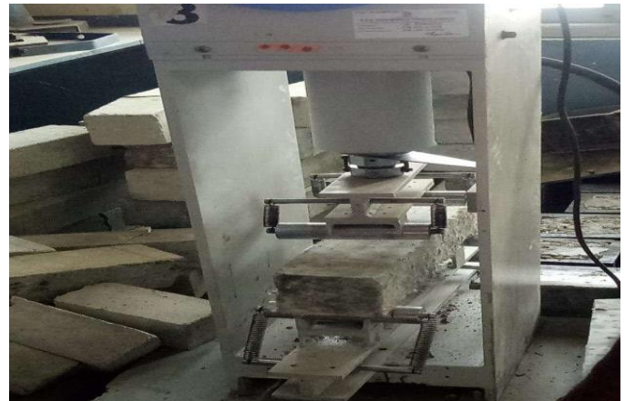
Fig -22: Placing Specimen for Loading
