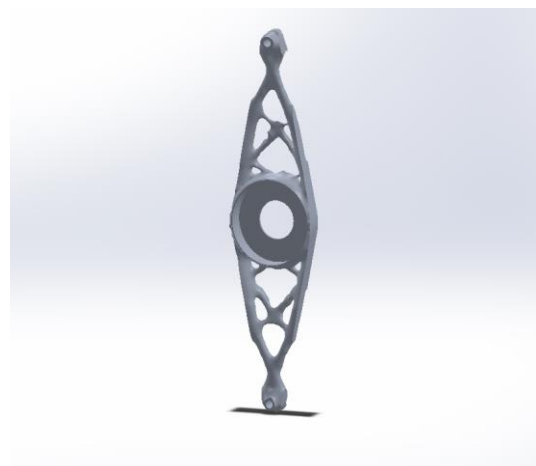
Figure 17- Topology Optimisation result
