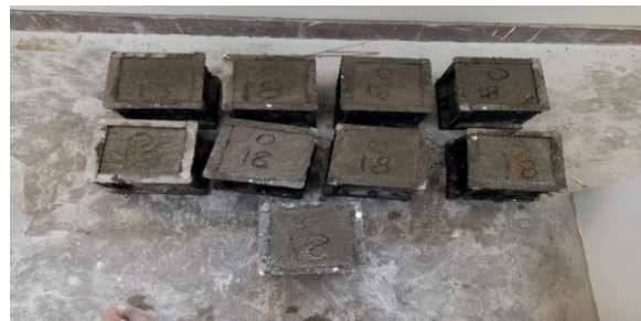
FIG-2 CONCRETE IN MOULDS
