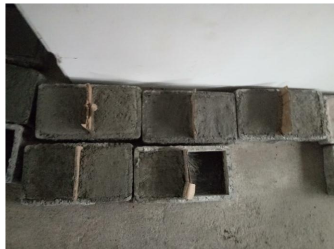
Fig-4: Compacted Papercrete
