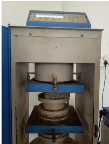
Fig-5: Compression of Papercrete
