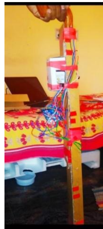
Fig -3: Integrating sensors on stick and encasing
