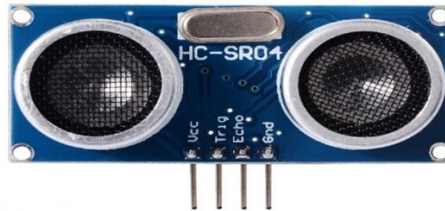
Fig: Ultrasonic Sensor (HC-SR04)
