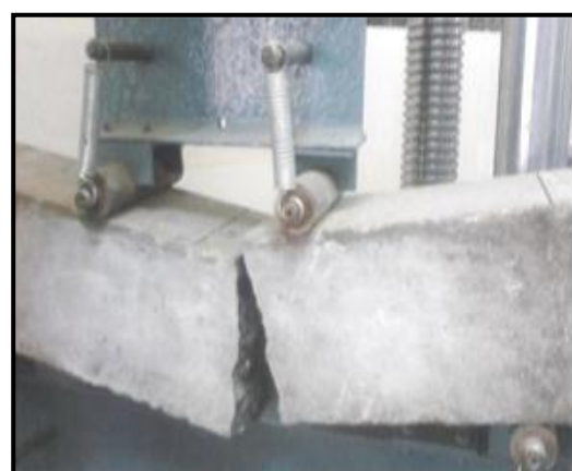
Fig-3: Testing of beam specimen in UTM
