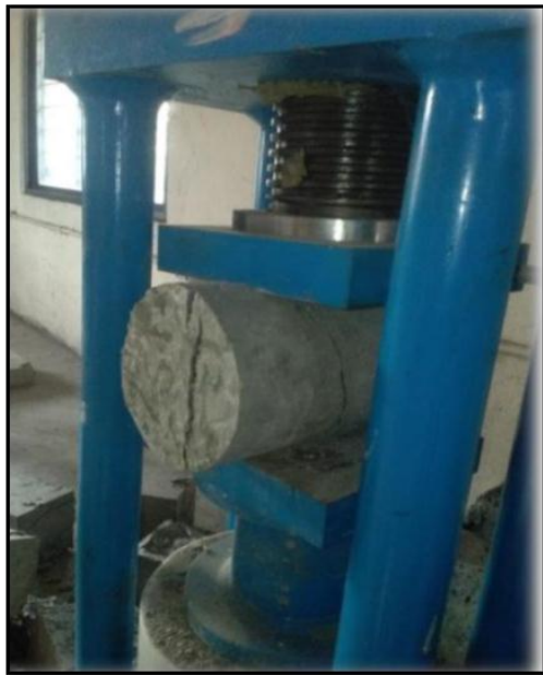
Fig-4: Testing of cylindrical specimen in CTM
