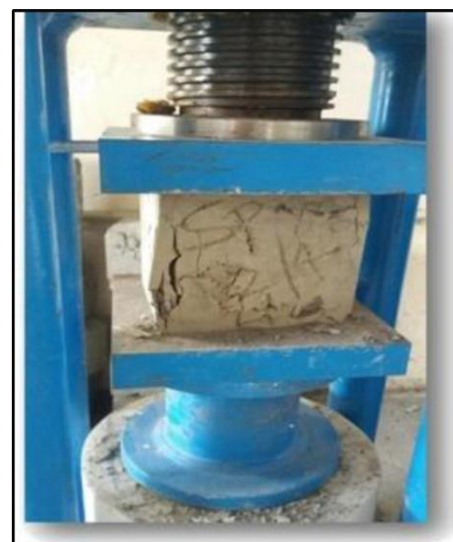
Fig-2: Testing of cube specimen in CTM
