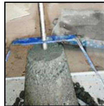
Fig-3: Testing of Slump using slump cone apparatus
