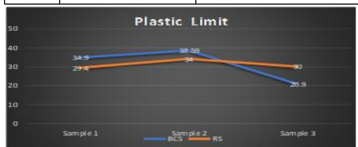
Chart No. 2 –Plastic Limit Determination
