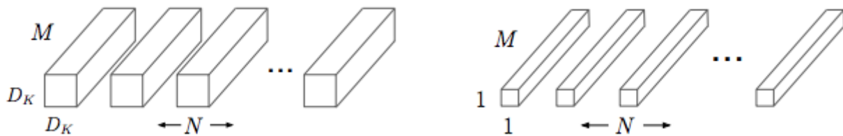
Fig -4.1: Standard convolutional filters [4] Fig -4.2: Depthwise convolution filters [4]
