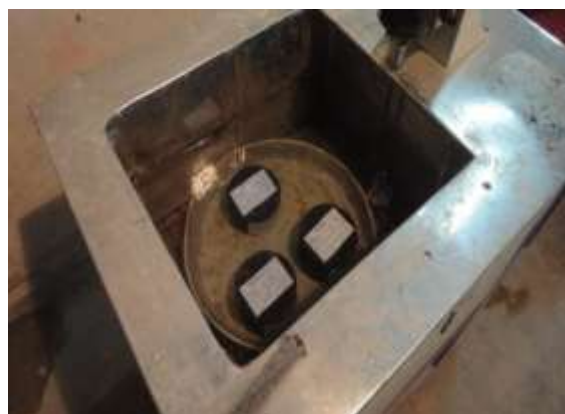
Fig 3 Marshall Samples in Thermostatically Controlled Water Bath
