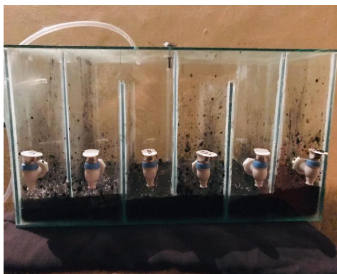
Fig -1: ABR reactor set up fed with raw sludge
