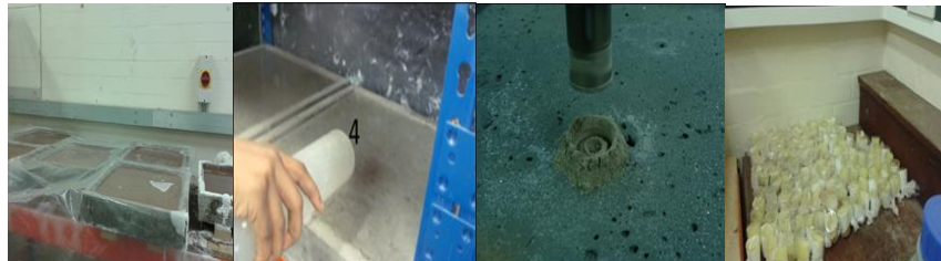
Fig.1 Cl - profile analysis in pre-conditioned concrete slabs
