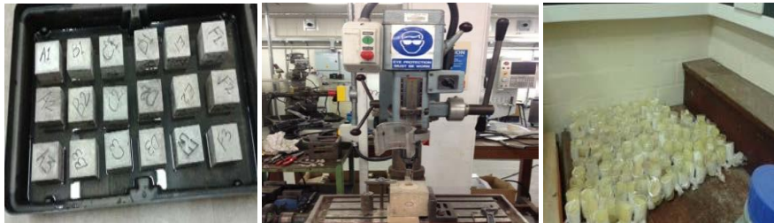
Fig.1 Cl- profile analysis in pre-conditioned concrete cubes
