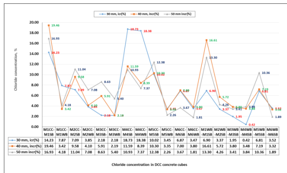
Fig.14 Cl - concentration in DCC concrete cubes
