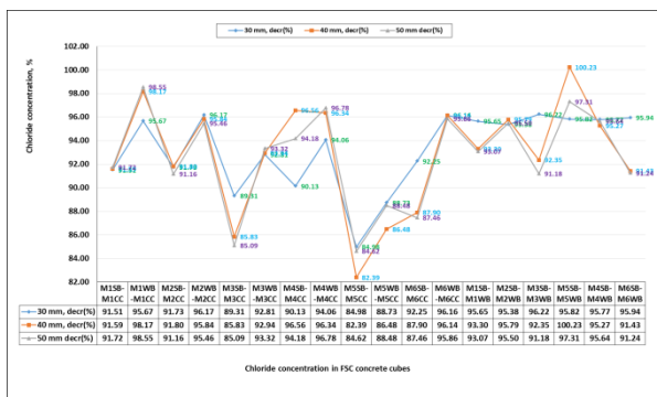
Fig.17 Cl- concentration in FSC concrete cubes
