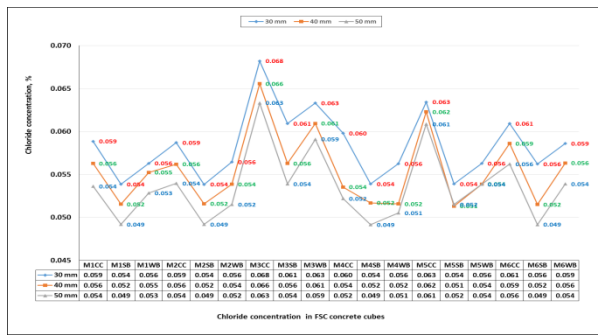
Fig.9 Cl - concentration in FSC concrete cubes
