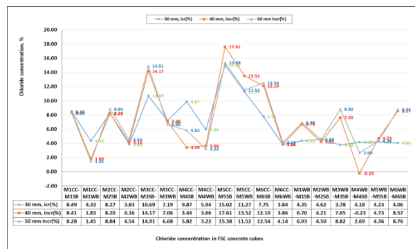
Fig.18 Cl- concentration in FSC concrete cubes
