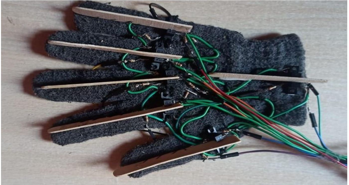
Fig.4(a)Prototype of hand glove with slot sensors
