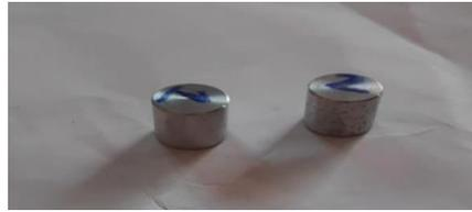
Figure 6: Hardness Tested Specimens
