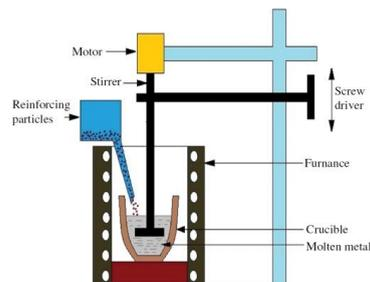
**Figure 1: Stir Casting Setup**
