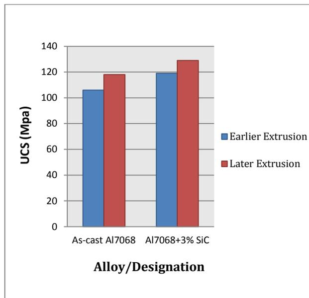
Figure 7: Compression test values of A7068 alloy and its composites earlier and later extrusion.
