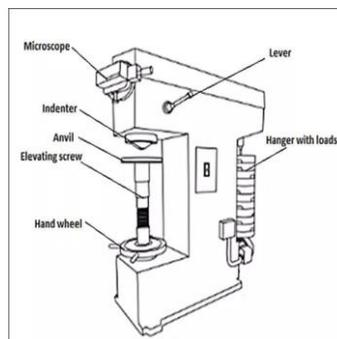
**Figure 3: Vicker Hardness Tester**
