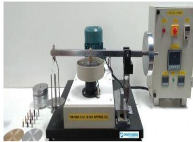
Figure 4: Pin-on-Disc Wear Machine
