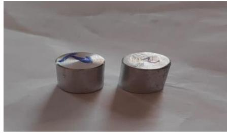
Figure 8: Compression Tested Specimens
