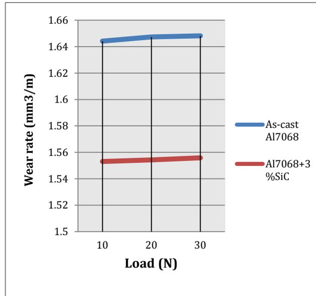
**Figure 10: Wear rate test values of A7068 alloy and its composites later extrusion.**
