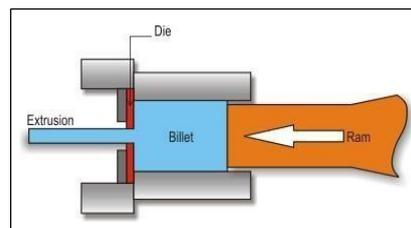
**Figure 2: Extrusion Setup**
